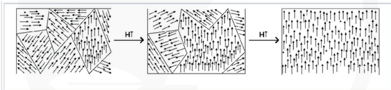
Figure 1. Rotation of direction and increase in size of magnetic domains in response to the externally applied magnetic field; Black arrow outside the box: the direction of the external magnetic field.
